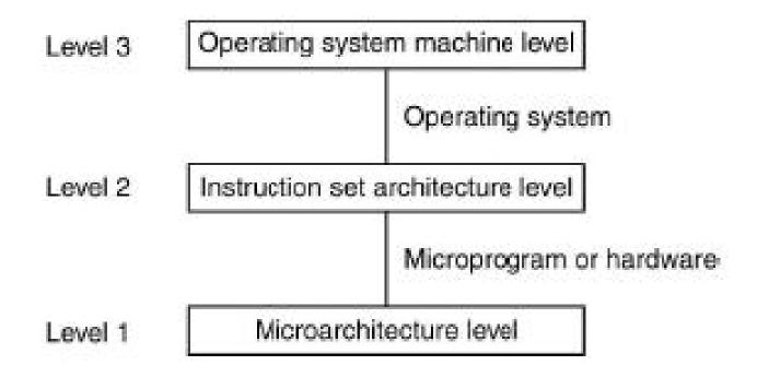
Positioning of the operating system machine level.
